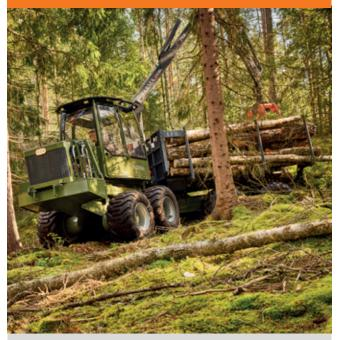
Optimized wheel speed, with full 8-wheel drive in forest work mode, results in less ground damage and less wear and tear on construction and transmission.
